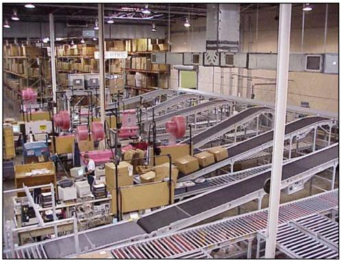
trol EZ-Logic conveyor accumulates the totes before the ship-sort system.
